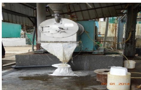
Salt separation through Pusher Centrifuge
